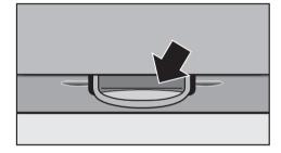
Also clean the small drip tray in the lower part of the inside of the front of the machine thoroughly.
